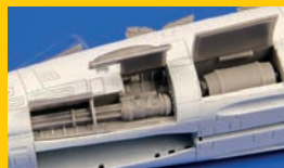
7453 F-14A Tomcat Port Side Cannon Installation
