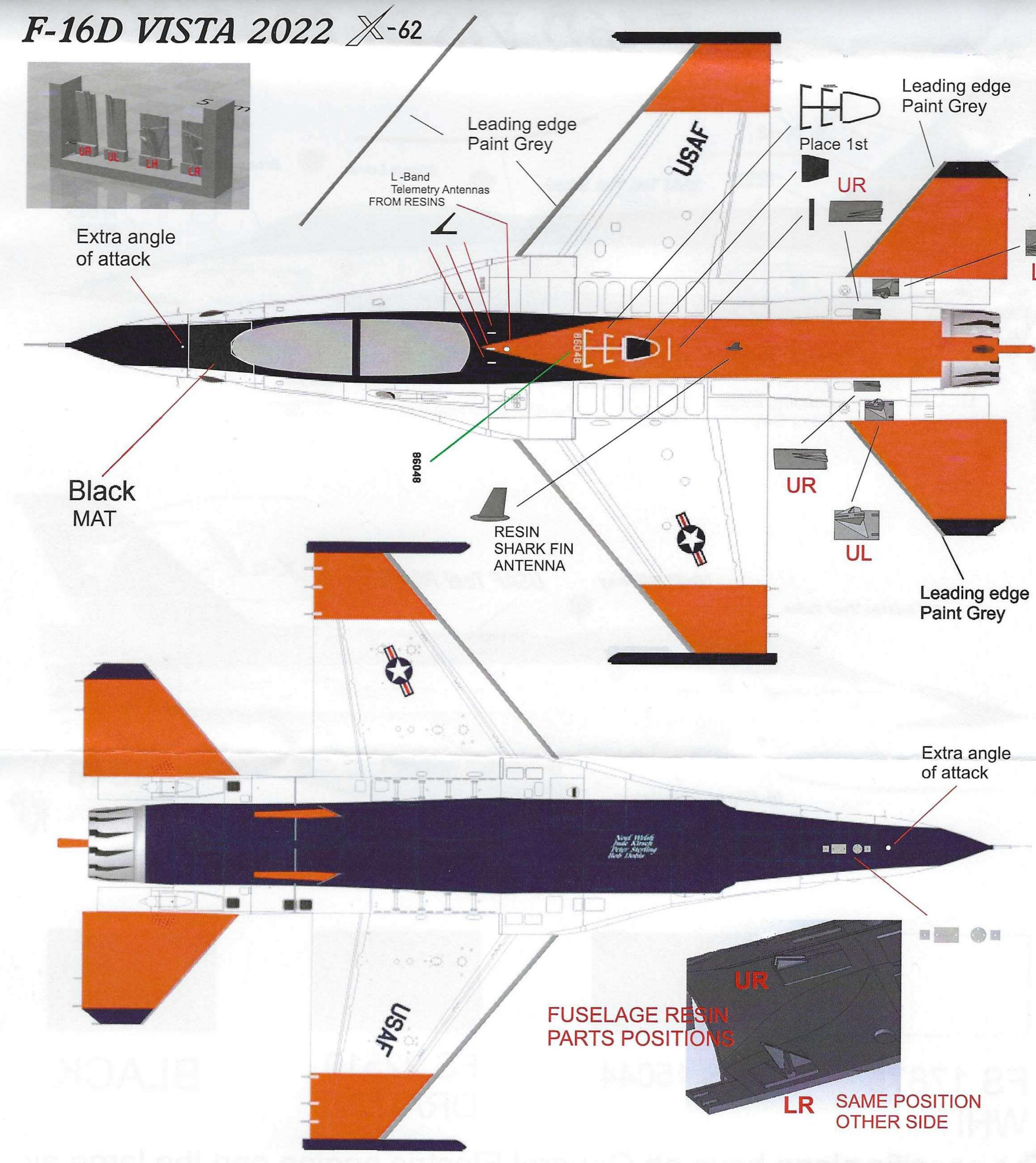
The VISTA is the only F-16 that equipped with 2 flight sticks in pilots cockpit. 1 on standard place and the 2nd between the pilots legs on the central console. Also has 4 ANGLES OF ATTACK probes 2 on standard positions, 1 on upper ane 1 on bottom of the radar cone
