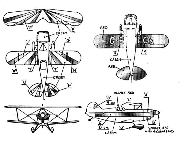
Should anyone wish to fit flying wires (model was not designed for this, but some people will try anything!) a length of fine Micro-rod is supplied. See sketch above assembly drawing for rigging positions. Spreader bars approx. 15mm long.
