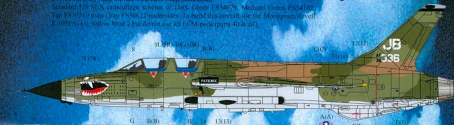
F-105G (Late) Thunderchief 63-8336 'PATIENCE' of 17th WWS/388th TFW, Korat RTAB, 1973. Standard US SEA camouflage scheme of Dark Green FS34079, Medium Green FS34102, Tan FS30219 over Gray FS36622 undersides. Note the Gray fin tip and Black band. To build this aircraft use the Monogram/Revell F-105F/G kit, use kit ECM fuselage pods (parts 40 & 67).
