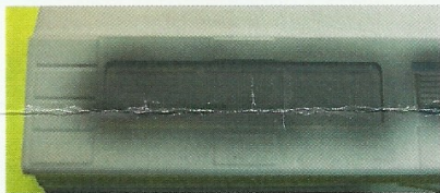
now prime the part and then paint the black window color over the whole area
