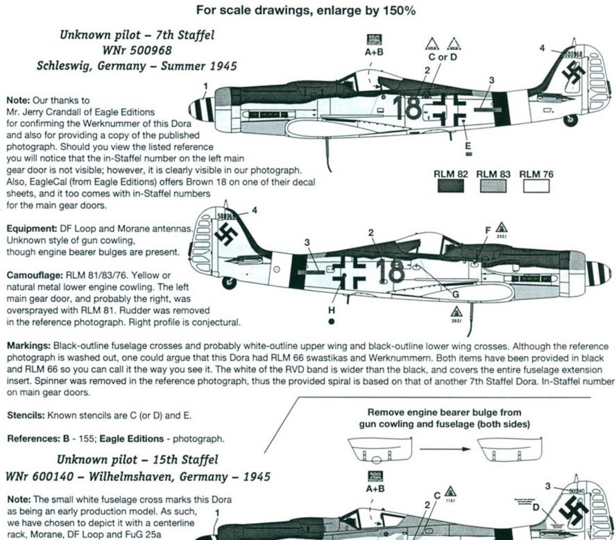
we have chosen to depict it with a centerline rack, Morane, DF Loop and FuG 25a antennas, and large swastikas. It appears that most of the original upper surface RLM 75 has been overpainted with RLM 83.
