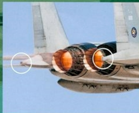
Asymmetric ECM Housings Specific to the F-15S
